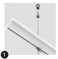
Mark and fix suspension kit mount point bodies onto ceiling using suitable screws into a beam, solid surface or strong fixing that is suitable for bearing weight.
